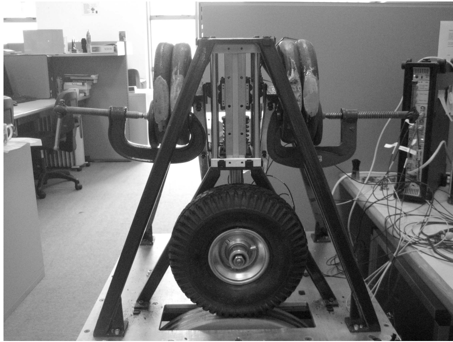
Figure 5.17: Quarter car rig with known added mass attached to the sprung mass
