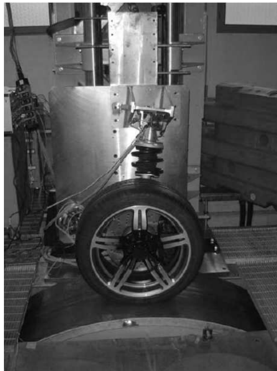
Figure 2.23: Ruotavia quarter car test rig (reproduced from [130])
