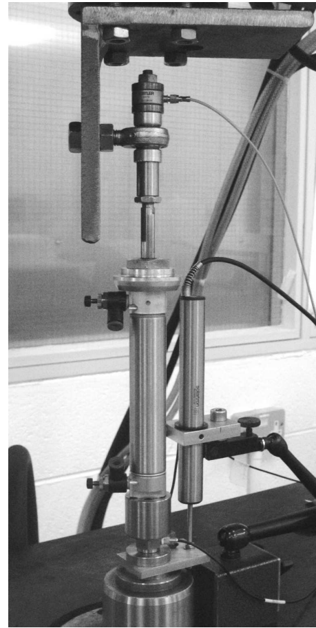
(b) Force measurement set-up mounted on the shock absorber during isolated testing
