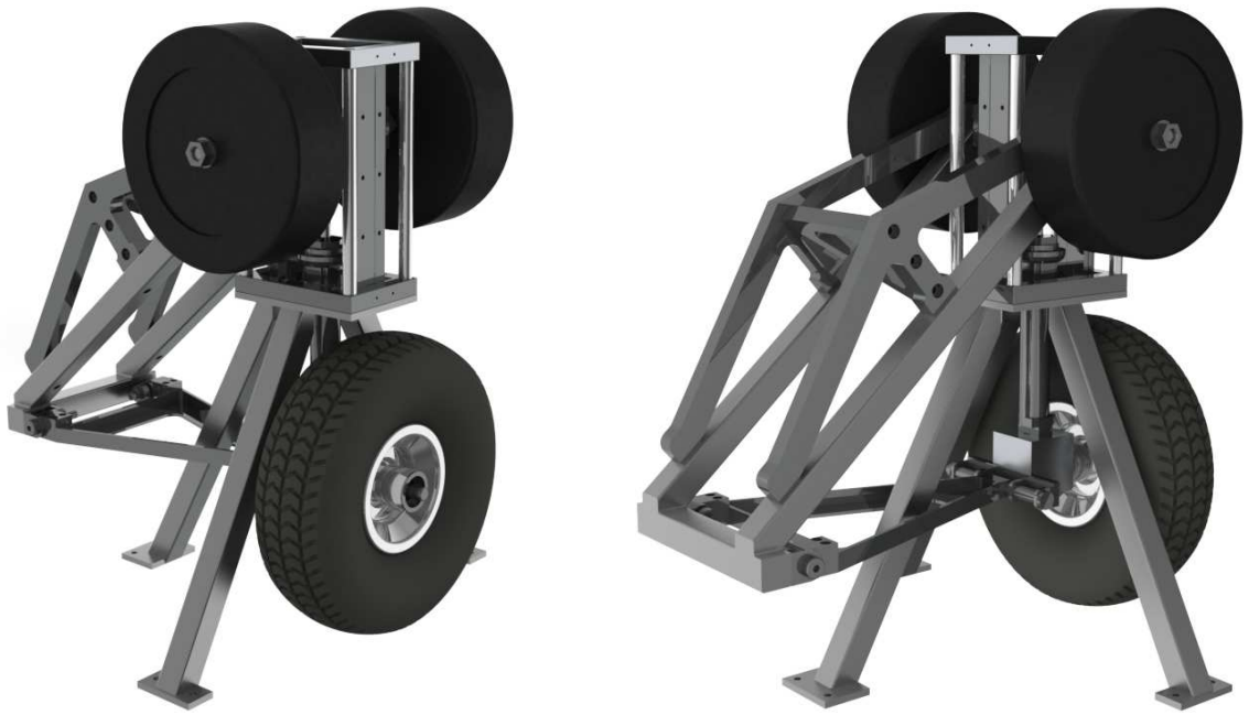
Figure 3.2: CAD drawings of the quarter car suspension experimental test rig showing the suspension system
