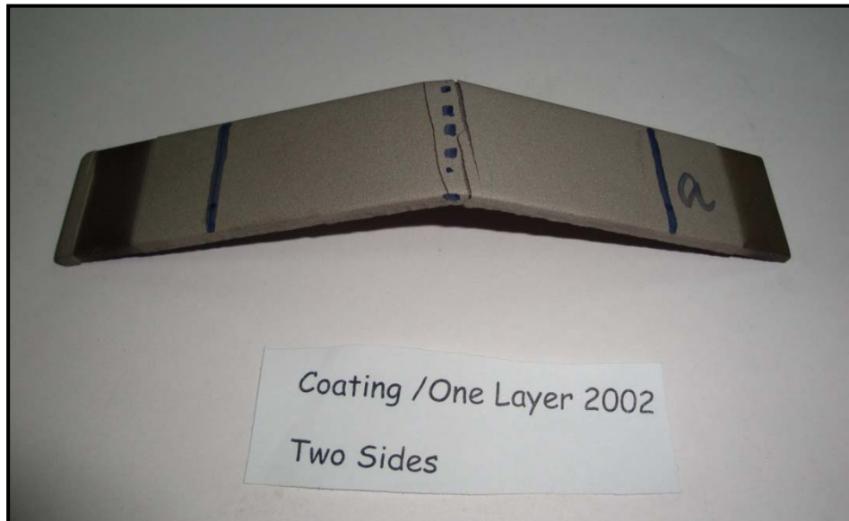
Figure 3.6 Workpiece after the three-point bending test
