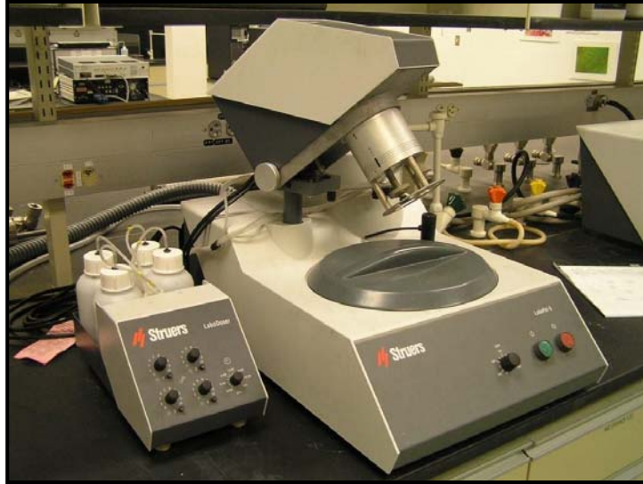
Fig 3.14 LaboPol 5 used for grinding and polishing
