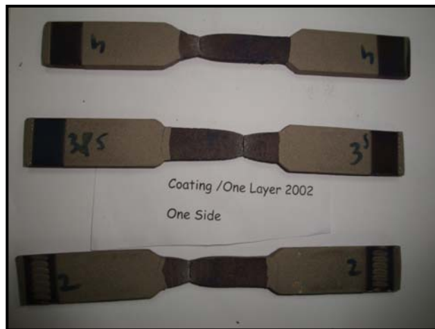
Figure 3.9 A photograph of work piece after the tensile test
