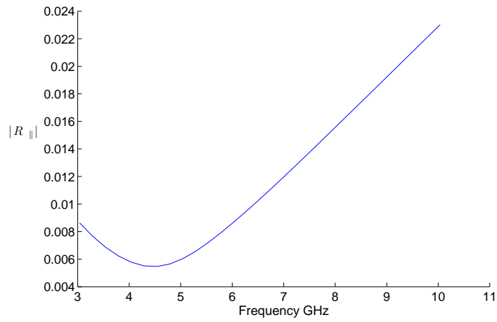
Figure 2.21: Variation of Parallel Reflection Coefficient R_{||} with Frequency at incident angle of 63^\circ
