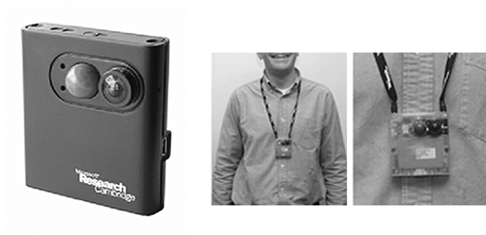
Figure 1. The Microsoft Sensecam, inset as worn by a user. (Adapted from Microsoft Research SenseCam homepage).
