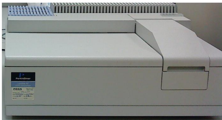
Fig. 2.12: Photograph of the Perkin Elmer Lambda 40 UV-Vis spectrometer.
