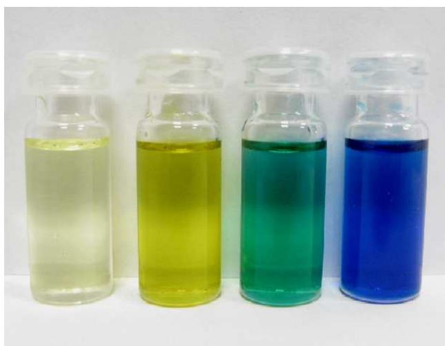
Figure 2.1: From left to right: IL, IL + \text{Cu}(\text{NO}_3)_2 (yellow), IL+ equimolar mixture (green) and IL + \text{Co}(\text{NO}_3)_2 (blue).
