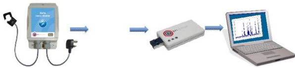
Figure 4 – A high-level overview of our in-home data gathering setup – the hardware setup.
