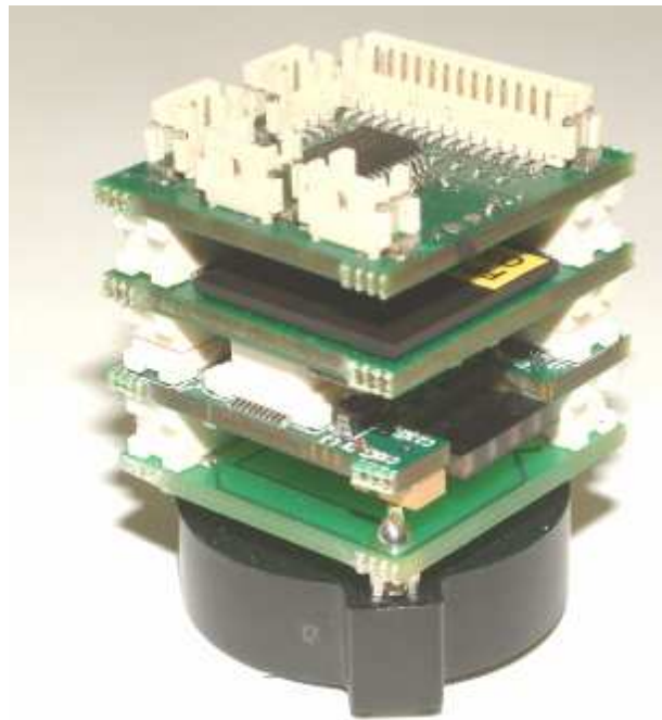
Figure 2: Our 25mm Modular WSN Prototyping Platform
