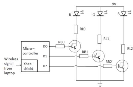
**Figure 4: Driving circuit used to control the RGB LED**
