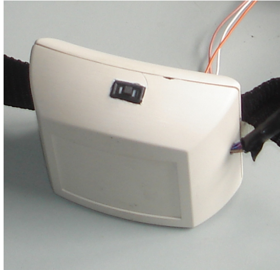
Figure 3.13: Battery powered digital phase fluorometry system in a belt-mountable housing.
