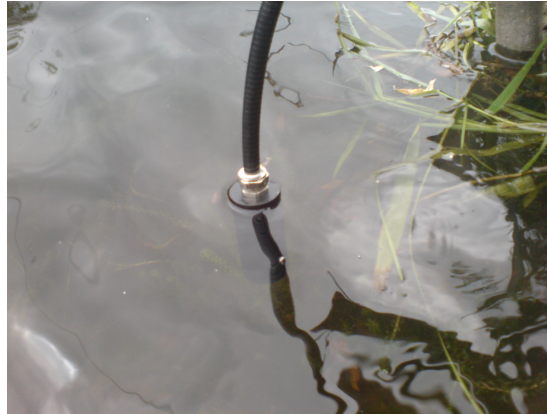
Figure 7.7: DO sensor in the field at a site on the River Liffey. The electronics enclosure, a battery pack and a laptop for logging the sensor data are located on the river bank. The flow velocity of the river was approximately 1m/minute
