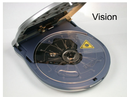
Fig. 1: Future vision of the Lab-CD platform: a portable player combined with an application specific, disposable disk [14].
