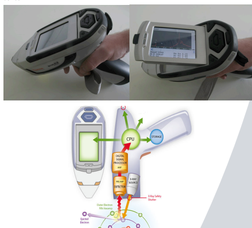
Fig. 3 The XRF handheld analyzer (left), The elemental composition is available immediately after measurement on the build in display (right). The XRF gun's principle of operation (bottom).
