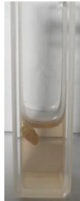
0.17mM o-dianisidine in buffer, 10 \mu l peroxidase enzyme, ionogel (-GOx) 40 \mu l of glucose (10% w/v)
