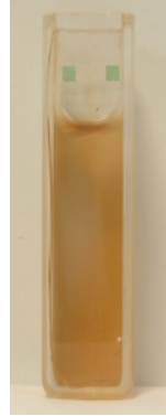
0.17mM o-dianisidine in buffer, 10 \mu l peroxidase enzyme, GOx ionogel 40 \mu l of glucose (10% w/v)
