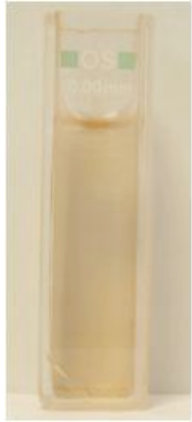
0.17mM o-dianisidine in buffer, 10 \mu l peroxidase enzyme GOx ionogel
