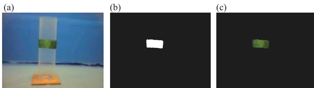
Figure 5. Segmentation process to selectively extract the pH indicator region of the test station in the water container. (a) Single captured image of a pH sensing station from the wireless camera. (b) Generated binary mask image after applying region segmentation image processing algorithms. White pixels representing the pH sensing strip region. (c) Resulting image of the extracted pH indicator region after applying the binary mask image to the original captured image.
