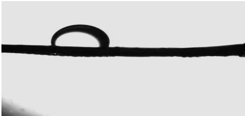
Figure 3.2.2 Pyro SS mesh at 0.5 mA/cm 2 for 90 minutes (control image)
