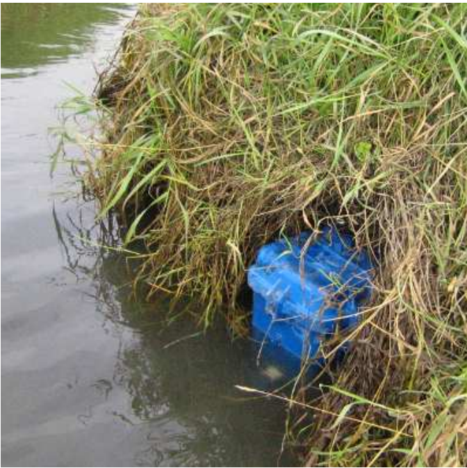
Fig. 3. The phosphate sensor in situ during the trial at Broadmeadow Water, Co. Dublin, Ireland in September 2009. The sample inlet is visible below the water line.
