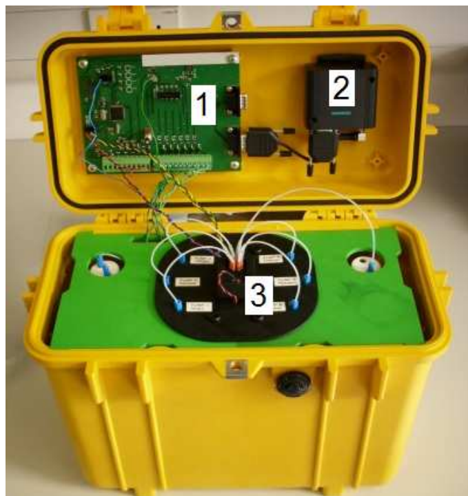
Fig. 1. The prototype phosphate analyser system. (1) Electronics board. (2) GSM modem. (3) Microfluidic chip / detector assembly. The battery, storage bottles, and solenoid pumps are contained within the lower part of the case.
