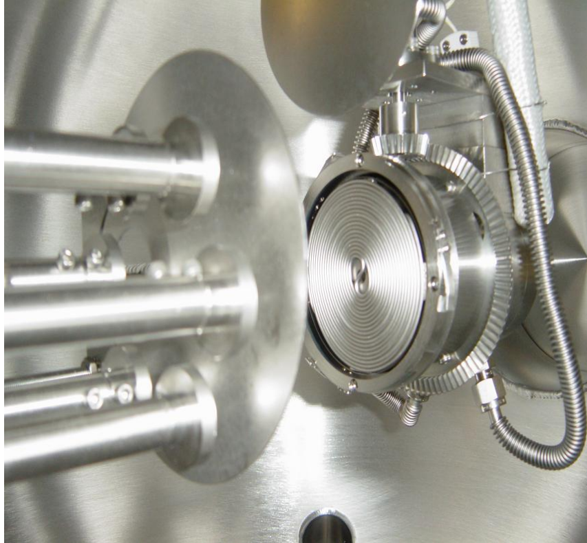
Figure 3.2: A close-up image of the heating unit and coils (without the nickel substrate disc). The target carousel and shield can be seen on the right hand side.
