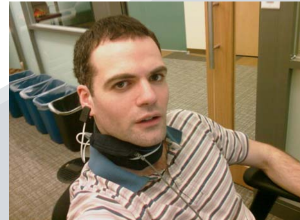
Sleep apnea neck cuff with oximeter, accelerometer, microphone, & gsr sensors
