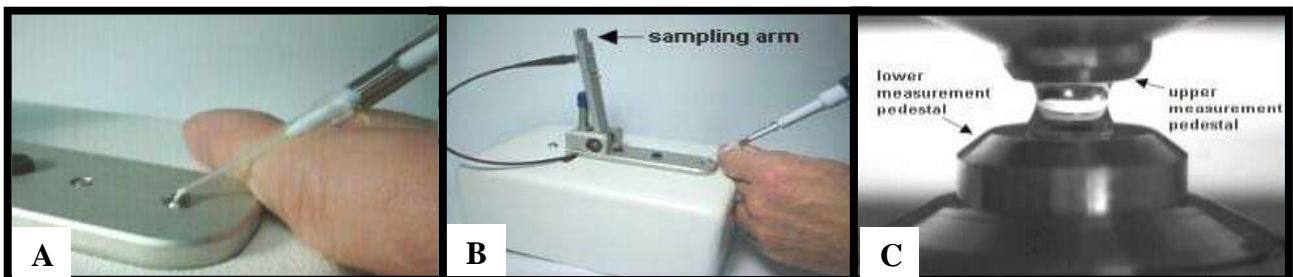
Fig 2.5.2.1: Samples are quantified by loading 1 \mu l onto the receiving fibre (A), the source fibre, connected to the sampling arm (B) is brought down into contact with the sample allowing a 1mm gap between the upper and lower pedestal (C), through which the light is passed. (Pictures adapted from ND-1000 Spectrophotometer users manual V 3.1.0).
