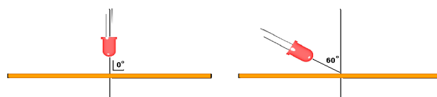
Fig. 2 Position of LED relative to the capillary during polymerisation
