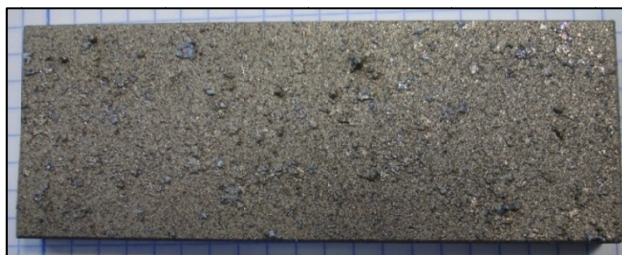
Figure 5.42. Visual aspect of Ti samples sprayed with the LEPS system
