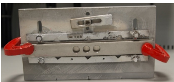
Figure 3.1. Three-hole die used to produce free-standing components
