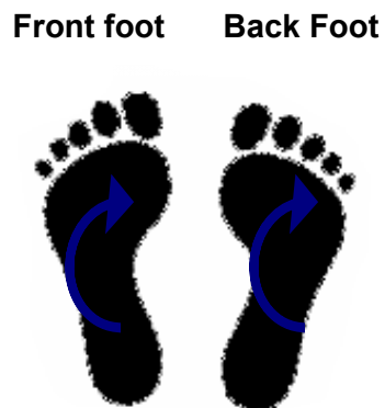
Figure 2.20 Definition of torque measurement by Worsfold et al. (2008). Positive rotation is movement to the lateral side of the back front and medial side of the front foot.
