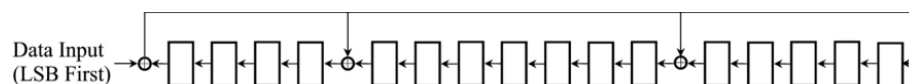
Figure 6: Hardware shift register described in IEEE 802.15.4 standard and used by the CC2420 chip.
