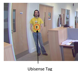
Fig. 3. UbiSense tag centered in the camera's field of view. The movement of the tag worn by the athlete is detected by the UbiSense infrastructure and its position calculated.
