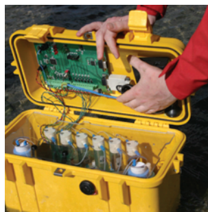
Figure 1: The phosphate analyser developed by CLARITY (left) and results over an 8-day period from a field trial at a waste water treatment plant (right) showing excellent agreement with a reference analytical system (total duration 49 days).
