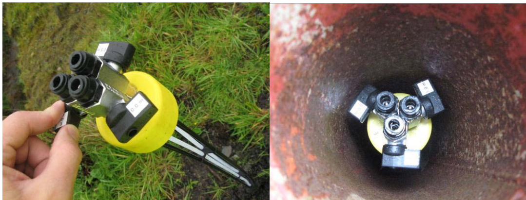
Figure 4 Multiple depth cap before insertion into borehole well and in borehole well
