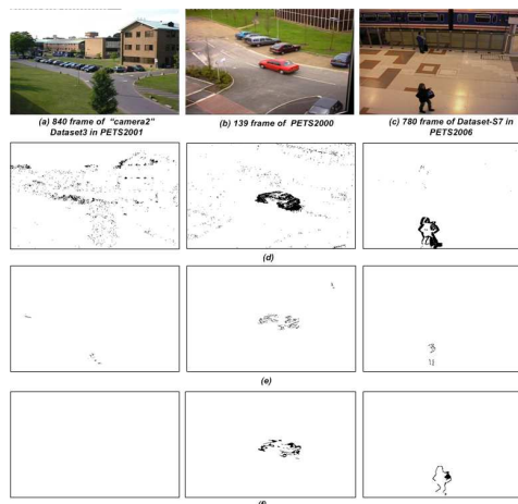
Figure 6: (a)(b) & (c) Sample test sequences used to illustrate performance for illumination changes, ghosting and fast moving objects; (d) results based on frame differencing, threshold ; (e) Chaohui's approach ; (f) the proposed method
