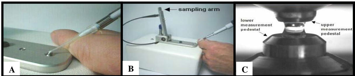
Fig: 2.5.1.4.1 Samples are quantified by loading 1 \mu\text{l} onto the receiving fibre (A), the source fibre, connected to the sampling arm (B) is brought down into contact with the sample allowing a 1mm gap between the upper and lower pedestal (C), through which the light is passed. (Pictures adapted from ND-1000 Spectrophotometer users manual V 3.1.0).
