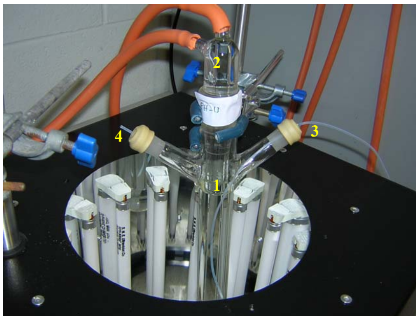
Picture 2: Rayonet photoreactor and experimental set-up ( 1: Pyrex reaction tube, 2: cold finger, 3: N 2 inlet, 4: gas outlet)
