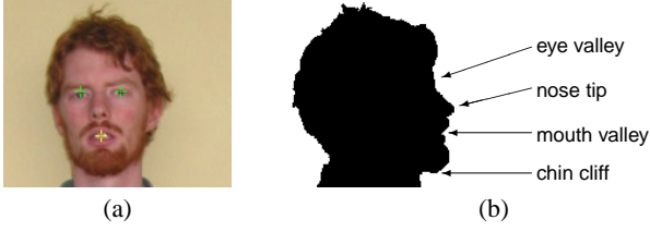
Fig. 4. Facial features locations in (a) front view and (b) side view head image.
