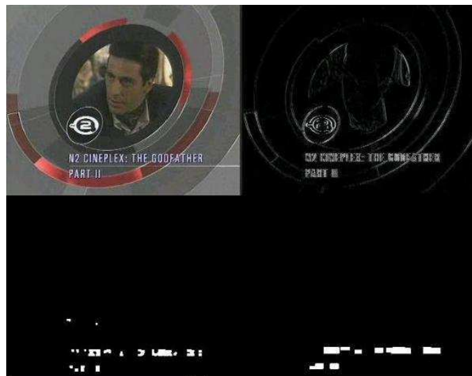
Figure A.3 (a) Input image, (b) horizontal difference magnitude, (c) (d) binarised edge map before and after morphological processing.
