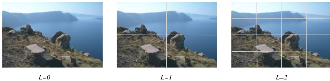
Figure 3-7: Illustration of the spatial pyramid scheme. The original image is from Vogel's dataset (Vogel and Schiele, 2004) and decomposed into two levels (middle and right). For each cell a separated histogram is computed.
