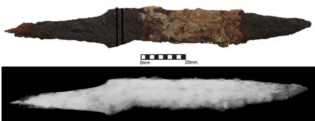
Figure 8.1: Photograph and x-radiograph of knife 12, the lines show where the section was removed.
