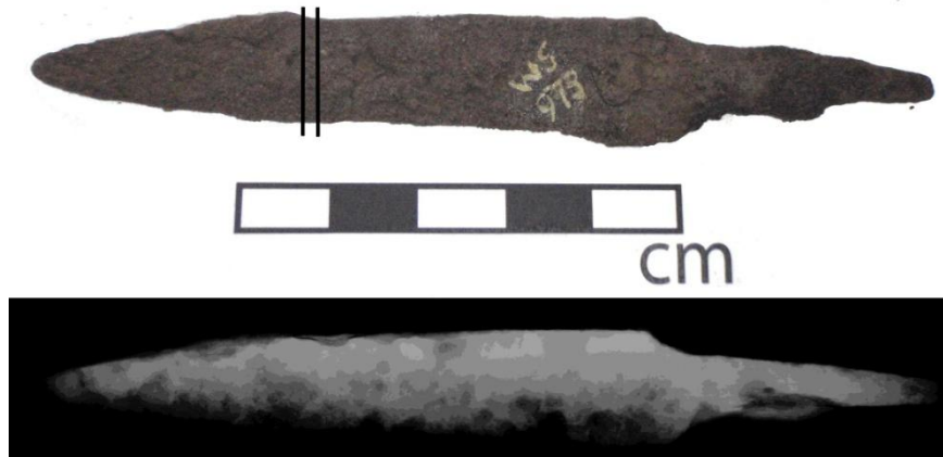
Figure 4.11: Photograph and x-radiograph of knife 973, the lines show where the section was removed.
