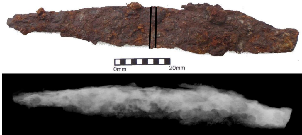
Figure 7.4: Photograph and x-radiograph of knife 116, the lines show where the section was removed.
