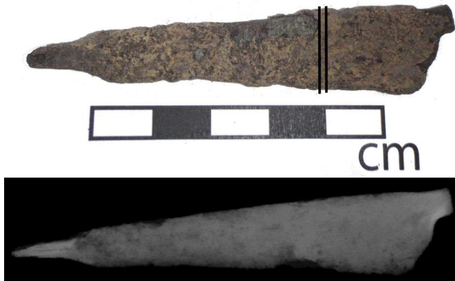
Figure 12.11: Photograph and x-radiograph of knife 1537, the lines show where the section was removed.
