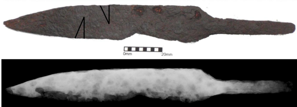
Figure 8.19: Photograph and x-radiograph of knife 257, the lines show where the sections were removed.
