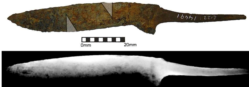
Figure 13.14: Photograph and x-radiograph of knife 14491, the lines show where the sections were removed.
