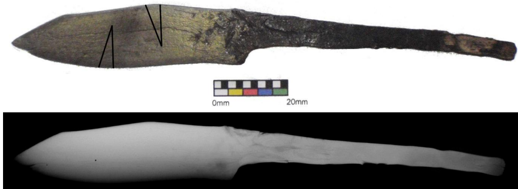
Figure 13.41: Photograph and x-radiograph of knife 604, the lines show where the sections were removed.
