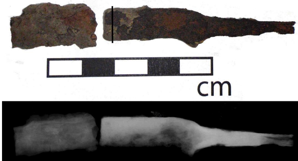
Figure 12.15: Photograph and x-radiograph of knife 84270, the line shows where the section was removed.
