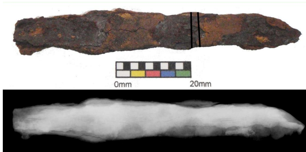
Figure 11.12: Photograph and x-radiograph of knife 429, the lines show where the section was removed.
