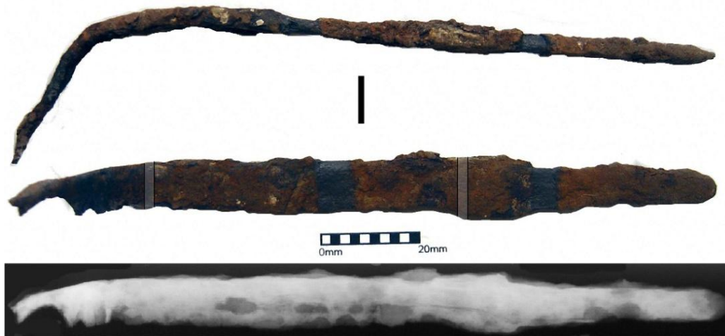
Figure 10.6: Photograph and x-radiograph of knife 75, the lines show where the sections were removed.
