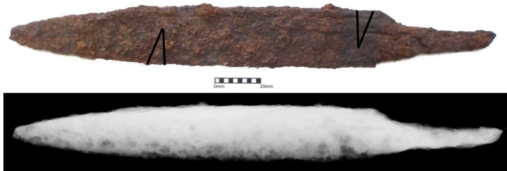
Figure 7.2: Photograph and x-radiograph of knife 103, the lines show where the sections were removed.
