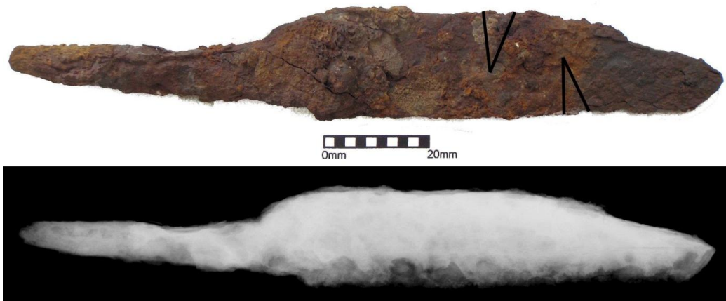
Figure 7.1: Photograph and x-radiograph of knife 100, the lines show where the sections were removed.
