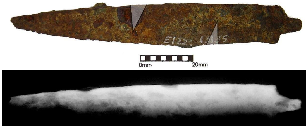
Figure 13.12: Photograph and x-radiograph of knife 13135, the lines show where the sections were removed.
