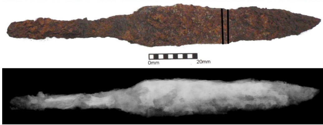
Figure 8.7: Photograph and x-radiograph of knife 118, the lines show where the section was removed.
