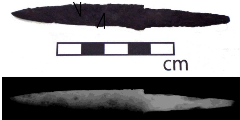
Figure 4.5: Photograph and x-radiograph of knife 433, the lines show where the sections were removed.
