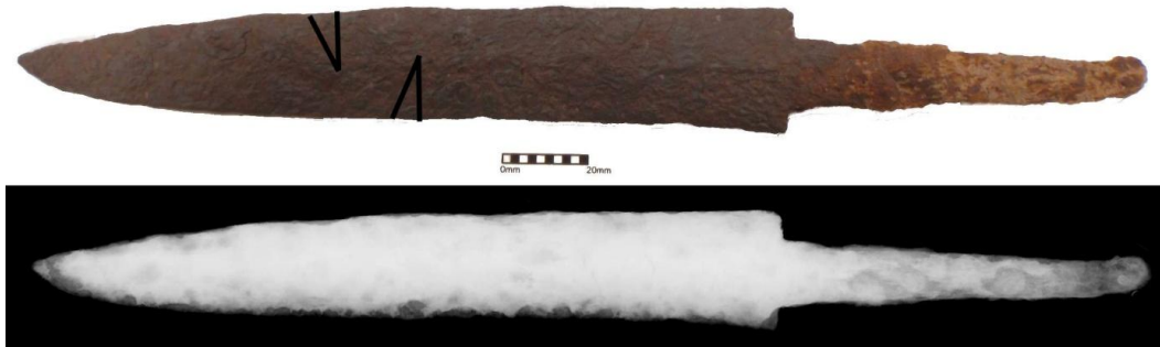
Figure 8.10: Photograph and x-radiograph of knife 175, the lines show where the sections were removed.
