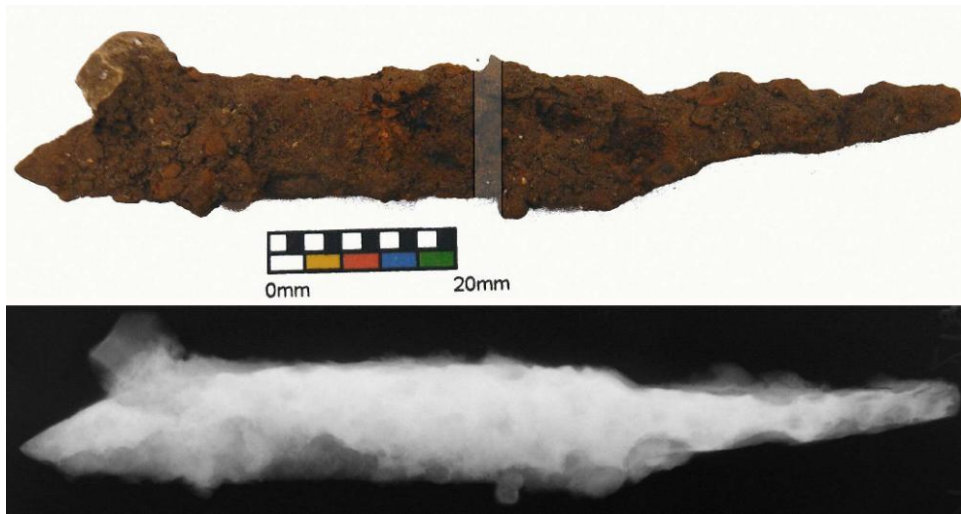
Figure 10.12: Photograph and x-radiograph of knife 218, the lines show where the section was removed.
