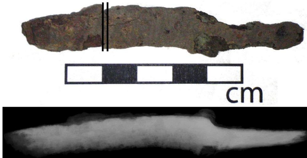
Figure 12.12: Photograph and x-radiograph of knife 1935, the lines show where the section was removed.
