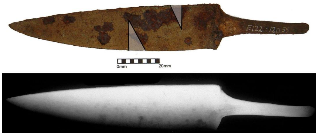
Figure 13.6: Photograph and x-radiograph of knife 12055, the lines show where the sections were removed.
