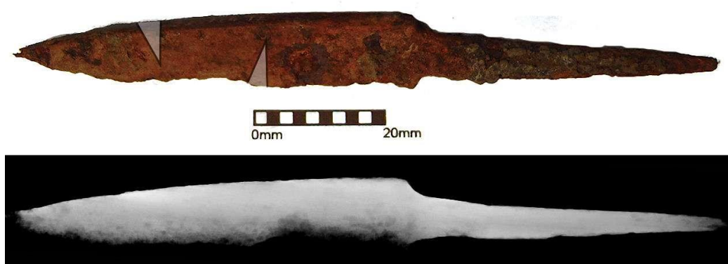
Figure 13.8: Photograph and x-radiograph of knife 12477, the lines show where the sections were removed.
