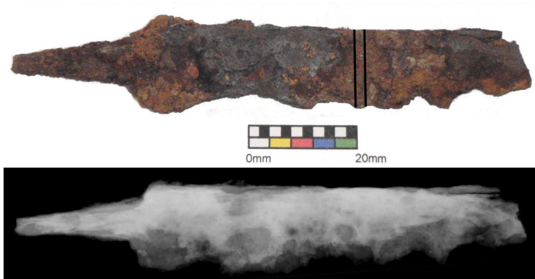
Figure 11.16: Photograph and x-radiograph of knife 1178, the lines show where the section was removed.
