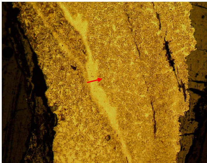
Figure 4.17: Line scan across the white weld line in West Stow Knife 973
