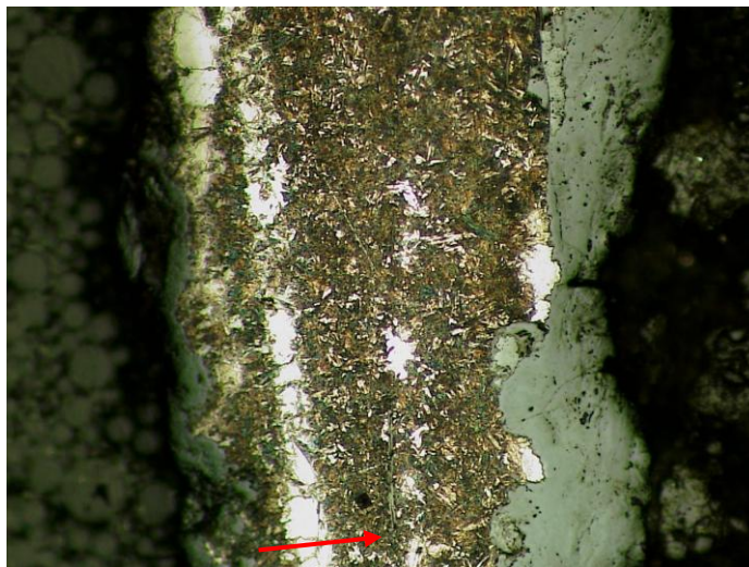
Figure 9.5: Line scan across another white weld line in Wharram Percy Knife 159
