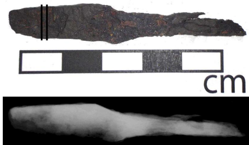
Figure 12.5: Photograph and x-radiograph of knife 84293, the lines show where the section was removed.
