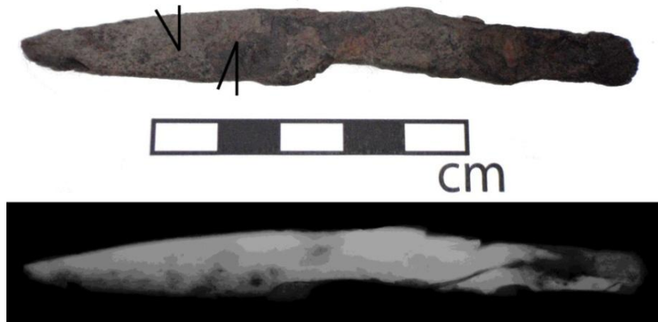
Figure 4.2: Photograph and x-radiograph of knife 86, the lines show where the sections were removed.
