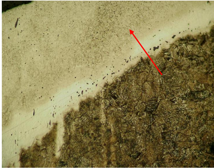
Figure 13.47: Line scan across the white weld line in Dublin Knife 13190
