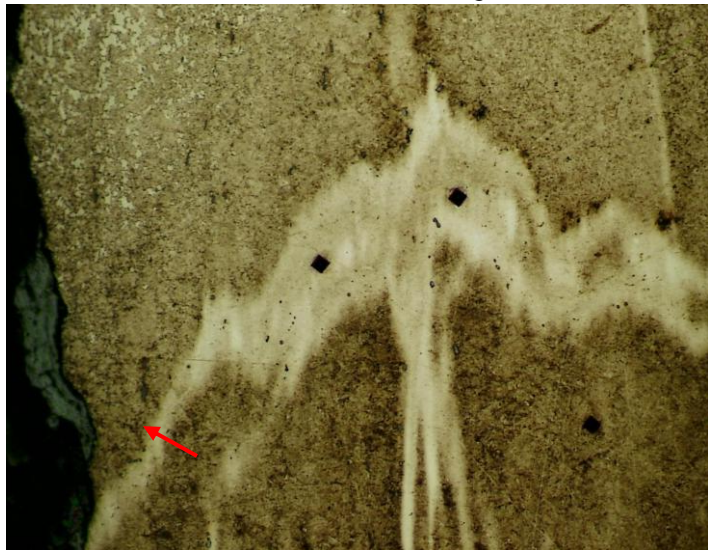
Figure 13.44: Line scan across the white weld line in Dublin Knife 323
