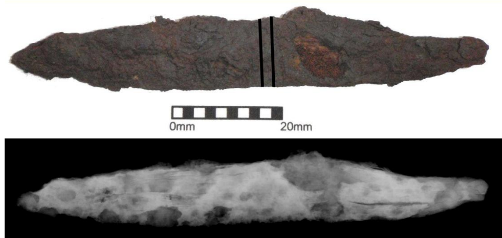
Figure 8.6: Photograph and x-radiograph of knife 116, the lines show where the section was removed.
