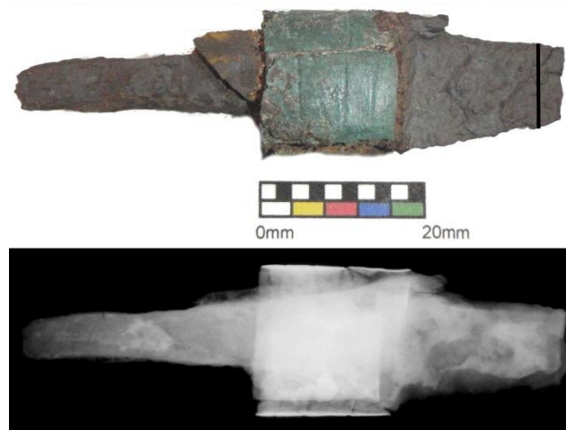
Figure 8.14: Photograph and x-radiograph of knife 217, the line shows where the section was removed.
