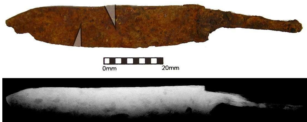
Figure 13.2: Photograph and x-radiograph of knife 6255, the lines show where the sections were removed.
