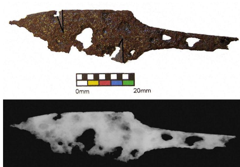
Figure 5.3: Photograph and x-radiograph of knife GM/M/53, the lines show where the sections were removed.
