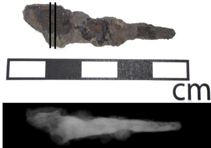
Figure 12.6: Photograph and x-radiograph of knife 1744, the lines show where the section was removed.
