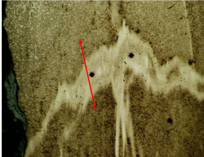
Figure 13.43: Line scan across the white weld line in Dublin Knife 323
