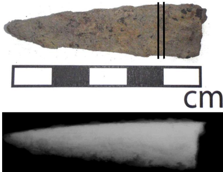
Figure 12.13: Photograph and x-radiograph of knife 11988, the lines show where the section was removed.
