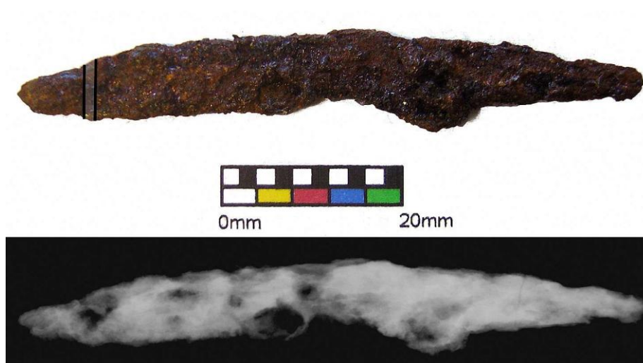
Figure 5.4: Photograph and x-radiograph of knife GM/M/61, the lines show where the section was removed.
