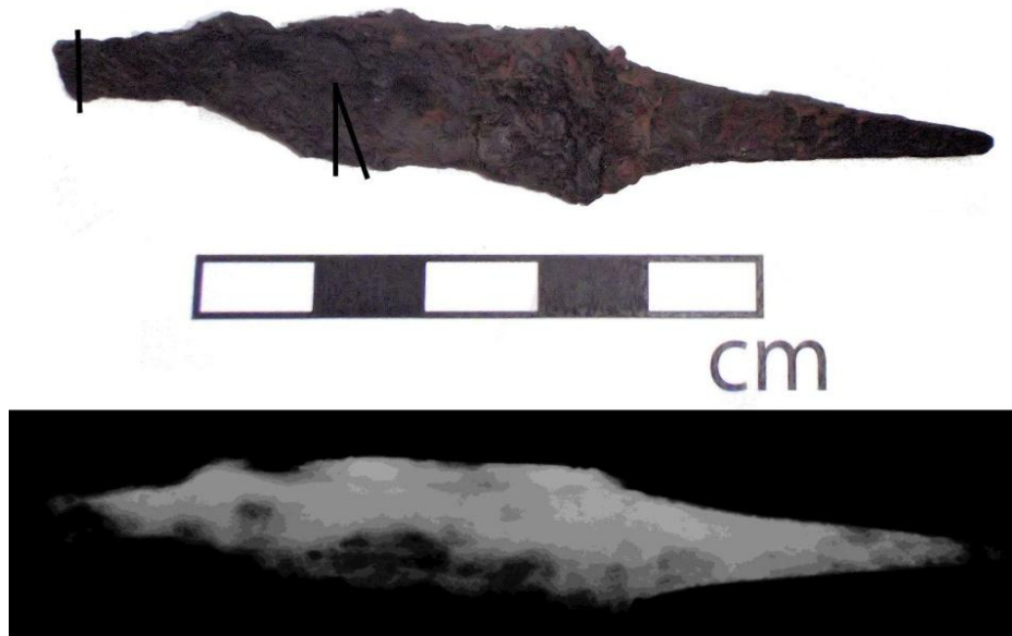
Figure 4.4: Photograph and x-radiograph of knife 330, the lines show where the sections were removed.
