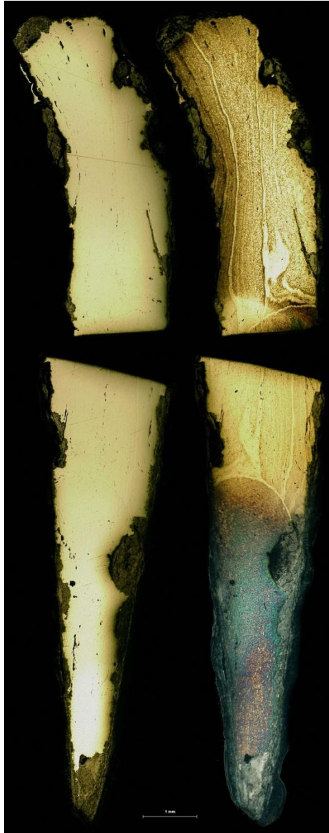
Figure 10.15: Mapped section of pivoting knife 4 in the un-etched (left) and etched condition (right).
