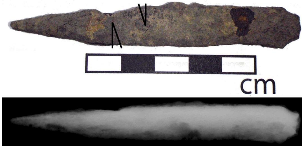
Figure 12.10: Photograph and x-radiograph of knife 813, the lines show where the sections were removed.
