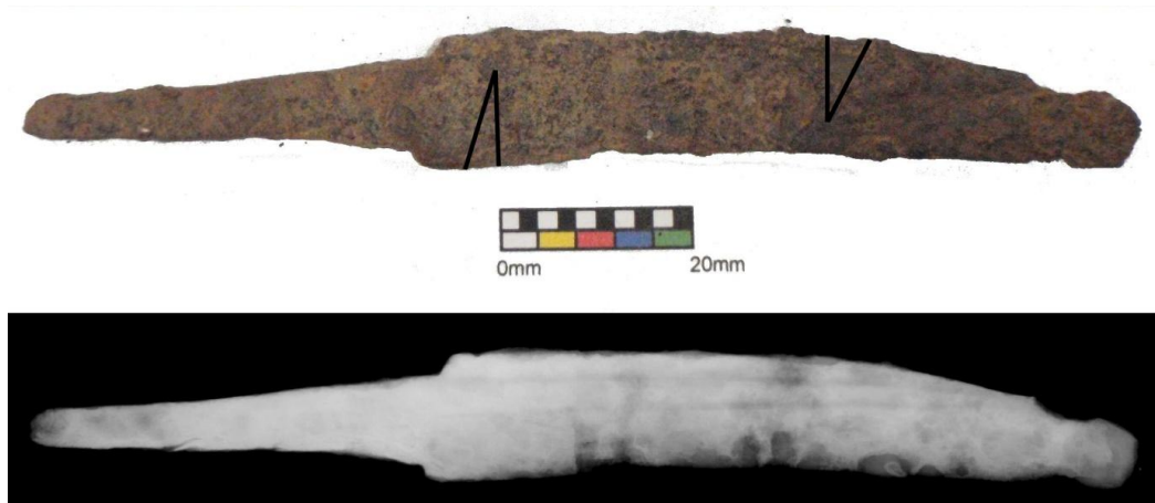
Figure 11.24: Photograph and x-radiograph of knife 3031, the lines show where the sections were removed.
