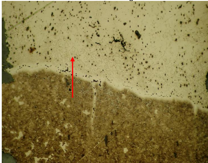
Figure 11.37: Line scan across the white weld line in Sedgeford Knife 3138
