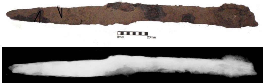
Figure 11.20: Photograph and x-radiograph of knife 2304, the lines show where the sections were removed.
