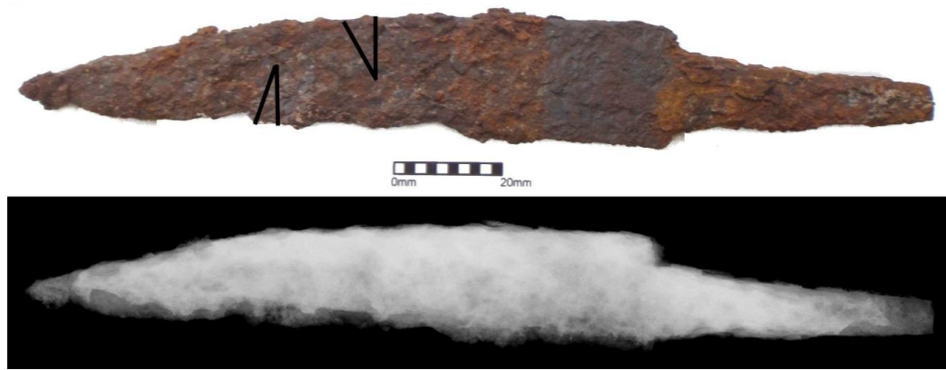
Figure 7.5: Photograph and x-radiograph of knife 127, the lines show where the sections were removed.
