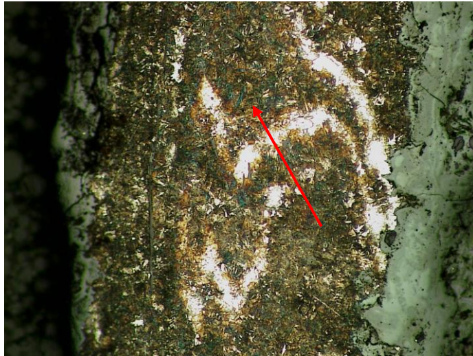
Figure 9.4: Line scan across two white weld lines in Wharram Percy Knife 159
