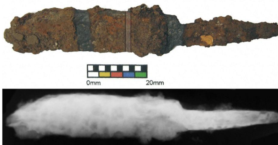
Figure 10.3: Photograph and x-radiograph of knife 67, the lines show where the section was removed.
