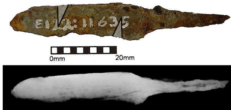
Figure 13.5: Photograph and x-radiograph of knife 11635, the lines show where the sections were removed.
