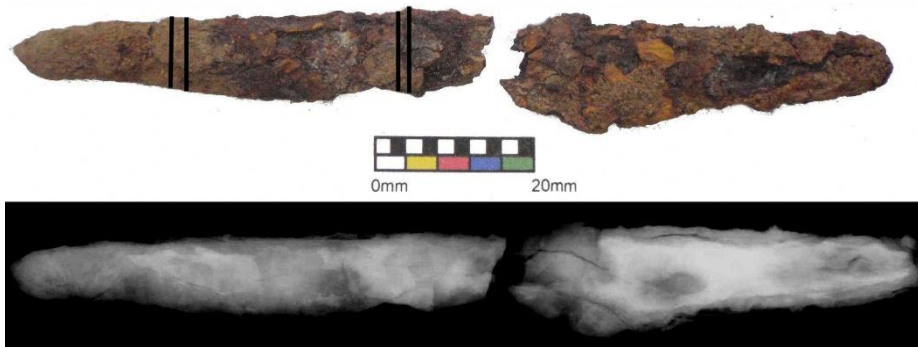
Figure 6.3: Photograph and x-radiograph of knife 11, the lines show where the sections were removed.
