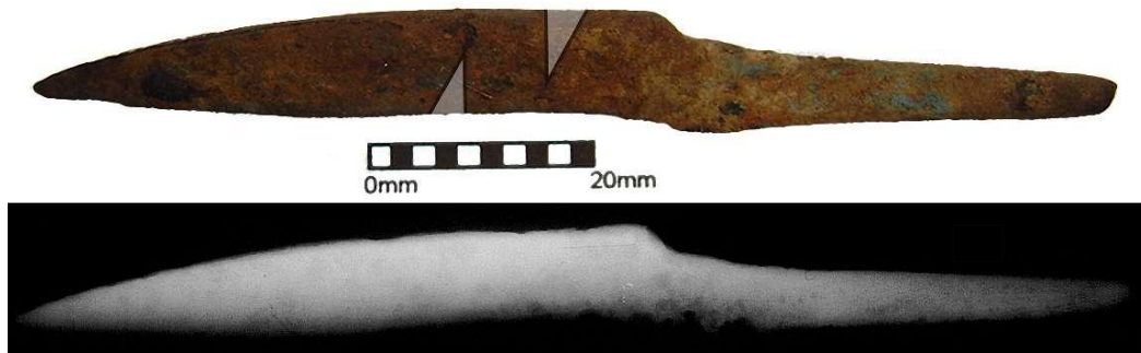
Figure 13.15: Photograph and x-radiograph of knife 15910, the lines show where the sections were removed.
