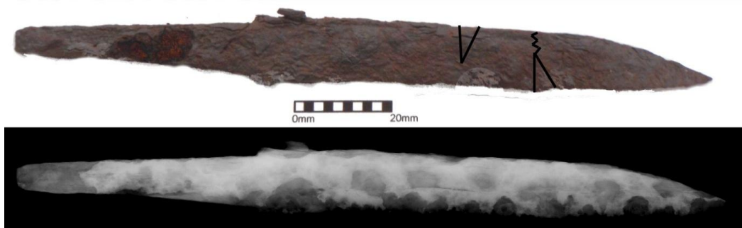
Figure 8.21: Photograph and x-radiograph of knife 266, the lines show where the sections were removed.
