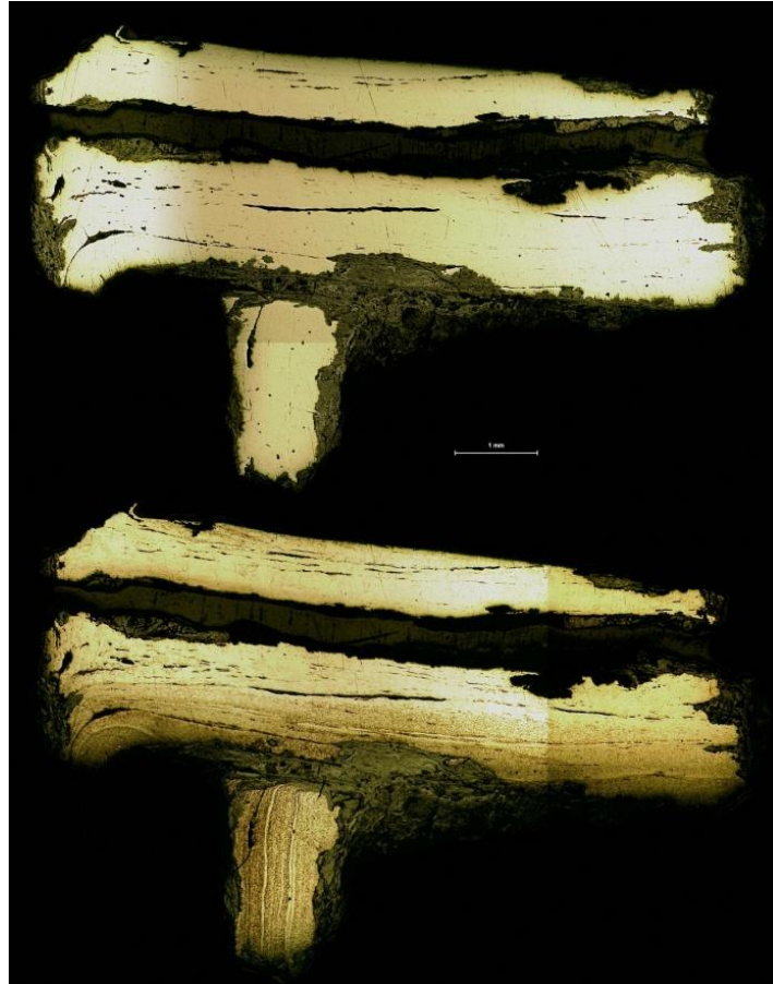
Figure 10.16: Mapped section of the pivot point in pivoting knife 4 in the un-etched (top) and etched condition (bottom).
