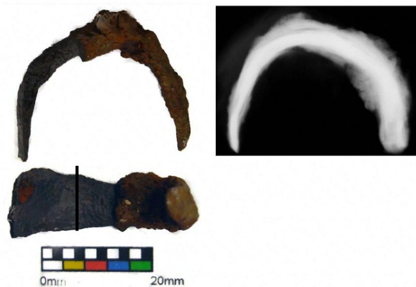
Figure 10.8: Photograph and x-radiograph of knife 113, the line shows where the section was removed.
