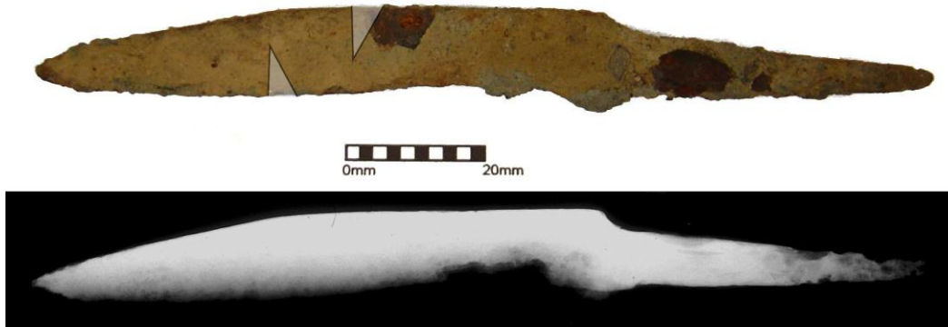
Figure 13.4: Photograph and x-radiograph of knife 8891, the lines show where the sections were removed.
