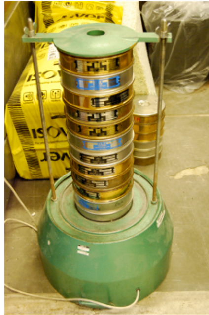
Figure 3.1: Experiment set up for sieve analysis
