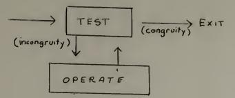
"The action is initiated by an 'incongruity' between the state of the organism and the state that is being tested for, and the action persists until the incongruity is removed."<sup>11</sup> The advantage of thinking of the feedback loop as a TOTE unit is that it can easily be applied to any hierarchial level by considering the "Operate" phase to include as many smaller TOTE units as is convenient for the inquiry.
