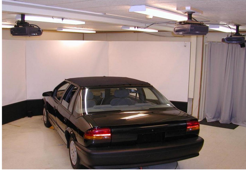
Figure 5. Driving simulator at Human Performance Laboratory, UMass Amherst
