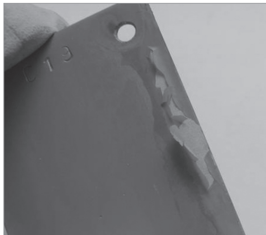
Figure 11 The flaky nature of the layer formed on pure copper after anodizing at 20V for 10 minutes
