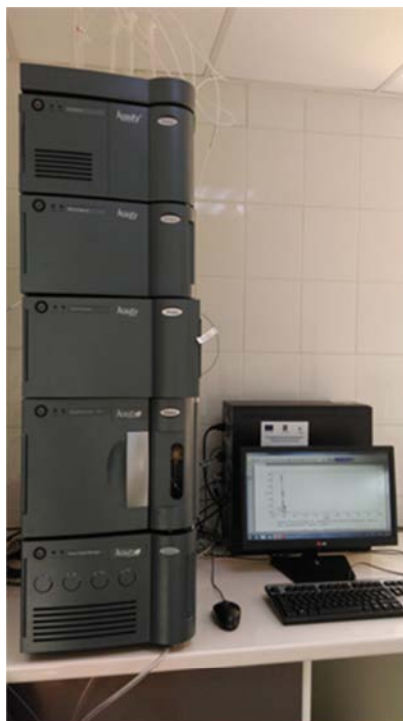
Figure 3. UPLC System Acquity equipped with Photodiode Array (PDA) and fluorescence (FLR) detector
