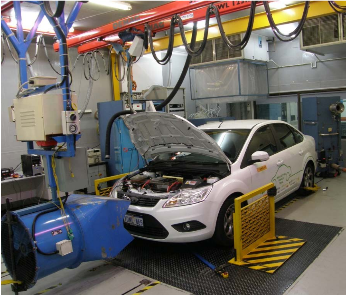
Figure 3: The Ford Focus EV on a chassis dynamometer under test conditions at Orbital's test facility.
