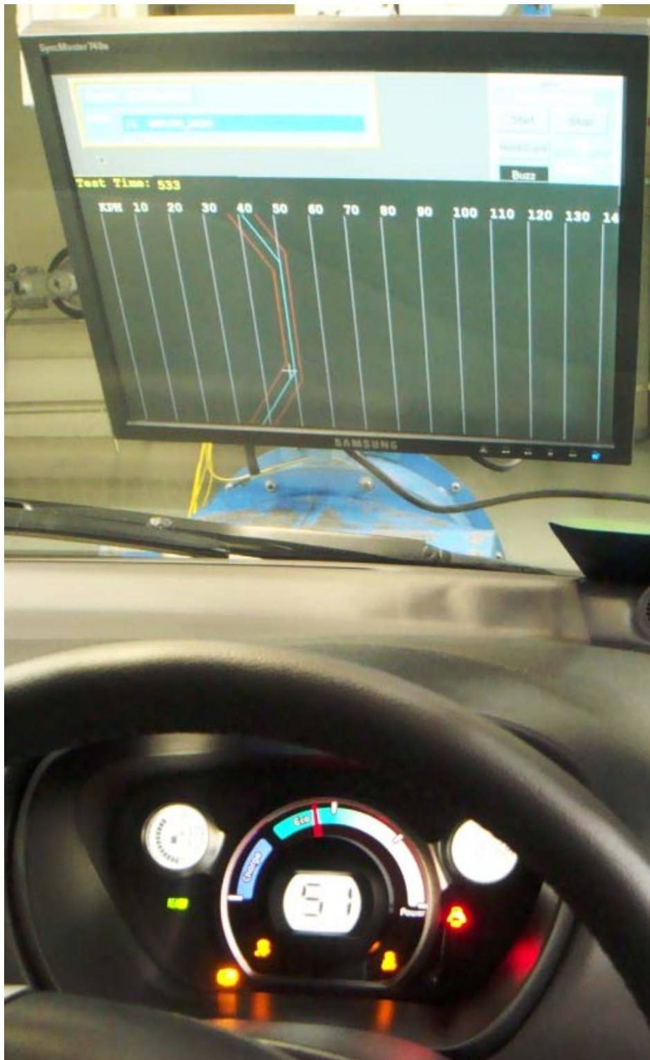
Figure 2: Computerised driving aid for a human test driver to follow a predefined drive cycle used during the testing at Orbital's facility. The blue line in the centre of the track is the indication of required speed to be driven. The red lines show the driver the maximum allowed speed deviation for a valid test drive, and the crosshair is the present speed. The uncertainty of the results can be inferred by the difference between the speed reading on the dashboard (51 km/h), and the crosshair (~49 km/h).
