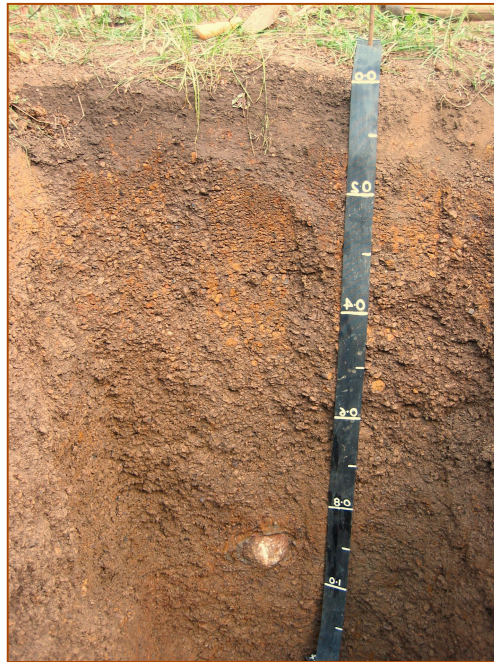
Fig. 4. Typical profile for Ou Reang Ov Soil group in Ou Reang Ov district, Kampong Cham province. Note the abundance of ferruginous gravel from about 15 cm depth and below, and the basalt rock at 90 cm depth.
