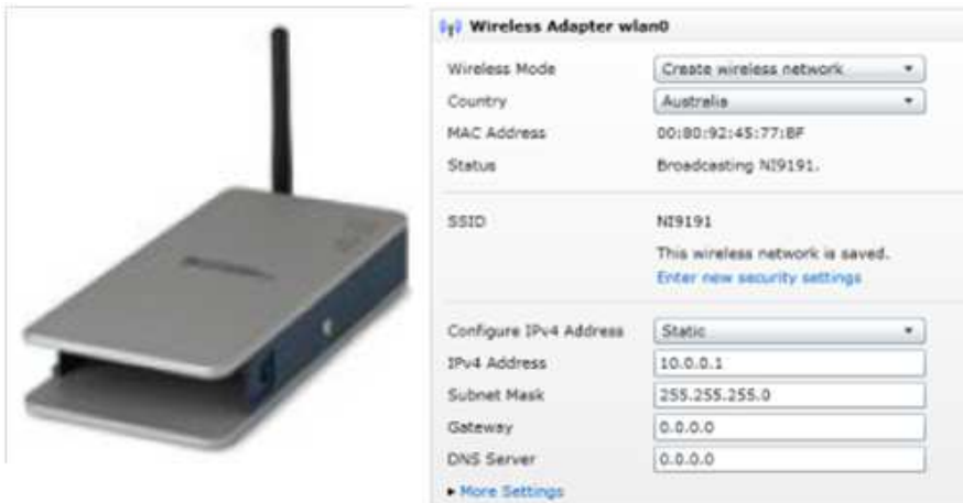
Figure 18 - (left) Picture of the cDAQ-9191 Wi-Fi module (Right) Network settings used to configure the connection (National Instruments 2010)
