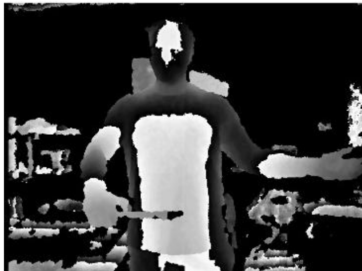
Figure 5: Depth Image produced by the calculations completed by the Microsoft Kinect Depth Sensor [23]
