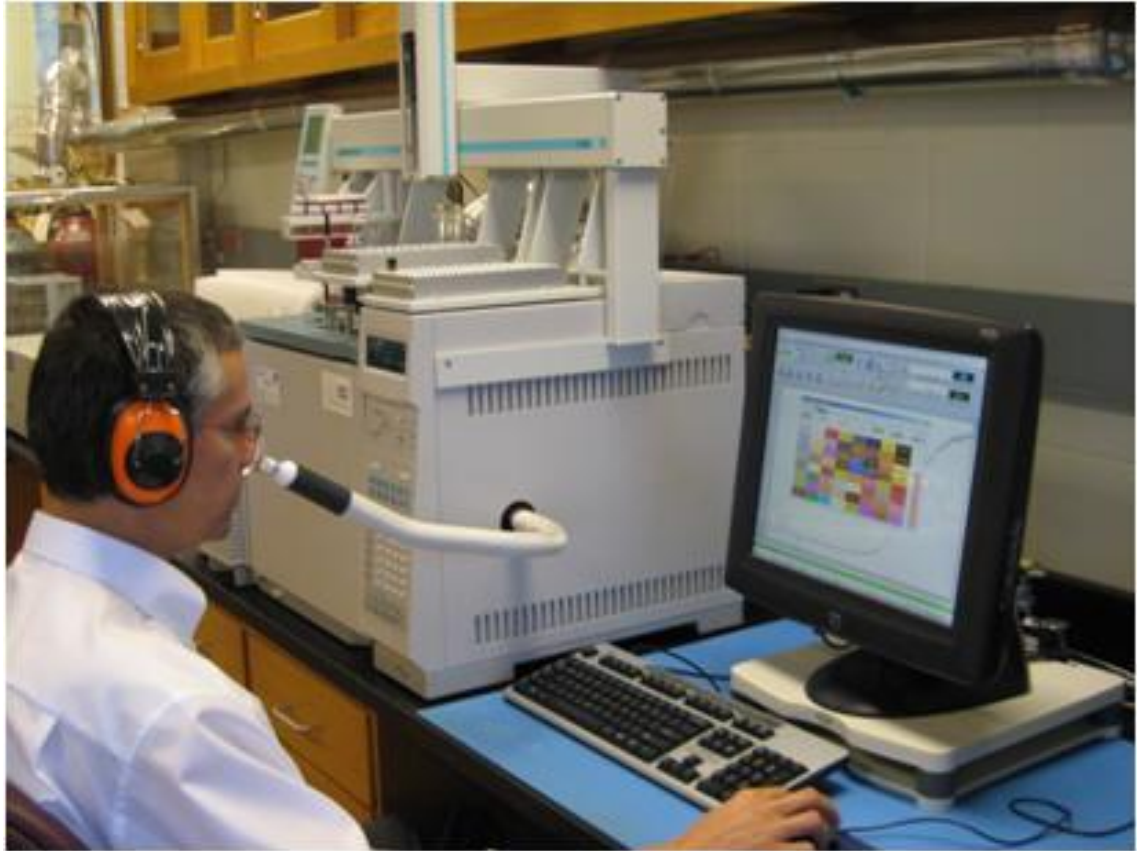
Fig. 1-3: Simultaneous GC-MS and olfactometry [36]
