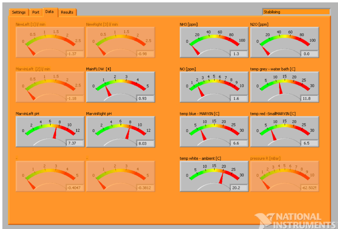
Fig. 3-11: Frontend MARVIN, visualization off 16 sensor readings
