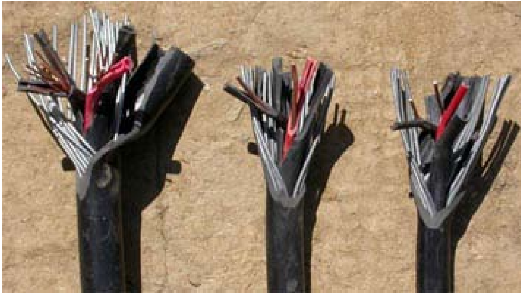
Fig 15: The three different sized, 4\text{mm}^2 , 2.5\text{mm}^2 , 1.5\text{mm}^2 , armored cables used in the Humla Solar PV systems.
