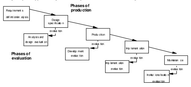
Figure 7.1. Mapping of the phases of a production process to corresponding evaluation phases
