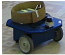
Fig. 5. Erratic with a mounted LRF Hokuyo
