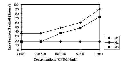
Fig. 1. Incubation period for the three media at different concentrations of faecal coliforms at 37°C Fig. 2. Incubation period for three media at different temperatures at a concentration of 160 CFU/100 mL
