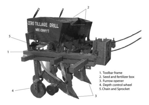
Fig. 8. The improved ACIAR-Rogro tined zero till seed drill (Photograph: R.J. Esdaile).
