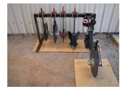
Fig. 10. A Bangladesh-made two-wheel tractor seed drill in strip tillage mode (Photograph: R.J. Esdaile).
