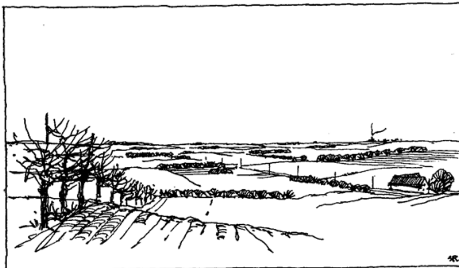
Figure 4.1: Illustration and description of terrain corresponding to roughness class 2 ( z_0 = 10m ) of the European Wind Atlas
