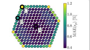
**Fig. 11** The MAE of the planar strain due to noise at each lattice point for a Wiener filtered noisy image at a sampling of 0.2 Å/pixel, a dose of  $10^3 e^-/\text{Å}^2$  and a defocus  $\Delta f = 8.5 \, \text{nm}$
