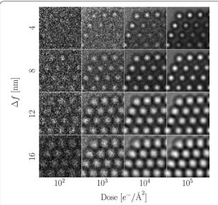
**Fig. 14** Sections of simulated HRTEM images for different doses and defocus at a sampling of 0.2 Å/pixel. All images are mapped onto the same range of greys
