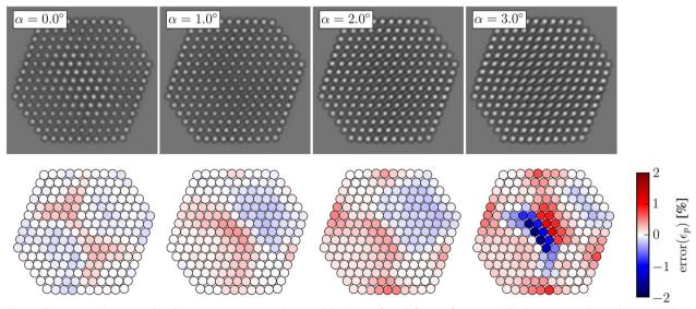
**Fig. 8** The top row shows simulated images at increasing tilt around the  $\Omega_{\text{T}}$  axis for a defocus  $\Delta f = 8.5$  nm. The bottom row shows the error in the planar strain at each lattice point measured from these images
