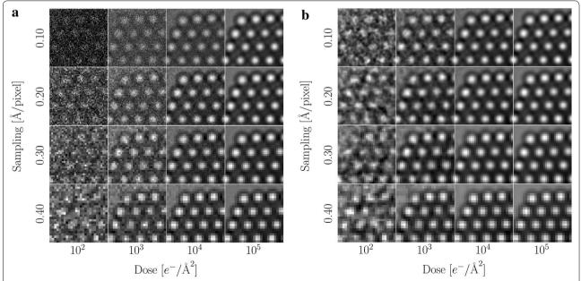
**Fig. 10 a** Sections of the simulated images at a defocus of  $\Delta f = 8.5$  nm for different doses and samplings. All images are mapped onto the same range of grey levels. **b** The same images after applying a Wiener filter
