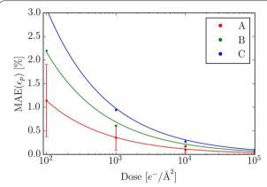
**Fig. 12** The MAE as a function of the dose for the three lattice points, *A*, *B* and *C*, as indicated in Fig. 11. The dots show the MAE calculated from the simulated images and the full lines are curves of the form given by Eq. (12), where the constant of proportionality has been fitted to the dots. The bars indicate the standard deviations, which for visual clarity are shown only for lattice point *B*, proportionally the standard deviations are similar for the other lattice points
