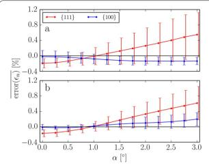
**Fig. 9** The error in the measured surface relaxations averaged across the facets as a function of tilt, around the axes (**a**)  $\Omega_1$  and (**b**)  $\Omega_2$ . The defocus was  $\Delta f = 8.5$  nm. The curves are for the {100} and {111} facets, as indicated by the legend
